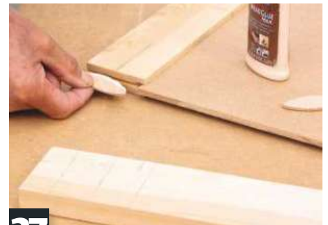
27 Dry assemble doors and adjust if necessary. After applying PVA glue on mating surfaces, insert biscuits in slots
